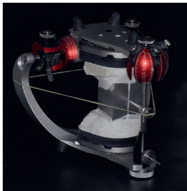
Fig 3 Mounting of the 3Shape occlusal transfer calibration object on the articulator.
